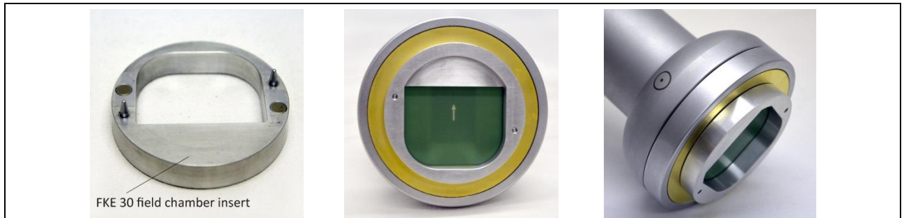
Figure 8: FKE 30 field chamber insert for use with P1202 field source
